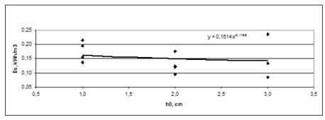
Fig. 4. Values of the specific energy  $E_s$  corresponding to the depth of cut  $h_0$
