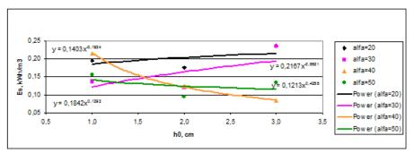
**Fig. 6.** Values of the specific energy  $E_s$ , corresponding to the depth of cut  $h_0$  for different values of the rake angle of the tooth -  $\alpha$
