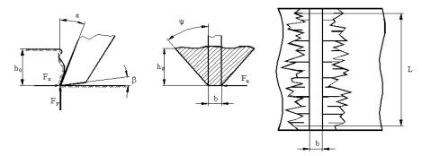
Fig. 1. Determination of the break-out angle  $\psi$
