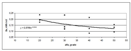
Fig. 5. Values of the specific energy  $E_s$  corresponding to the rake angle of the tooth -  $\alpha$ ,
